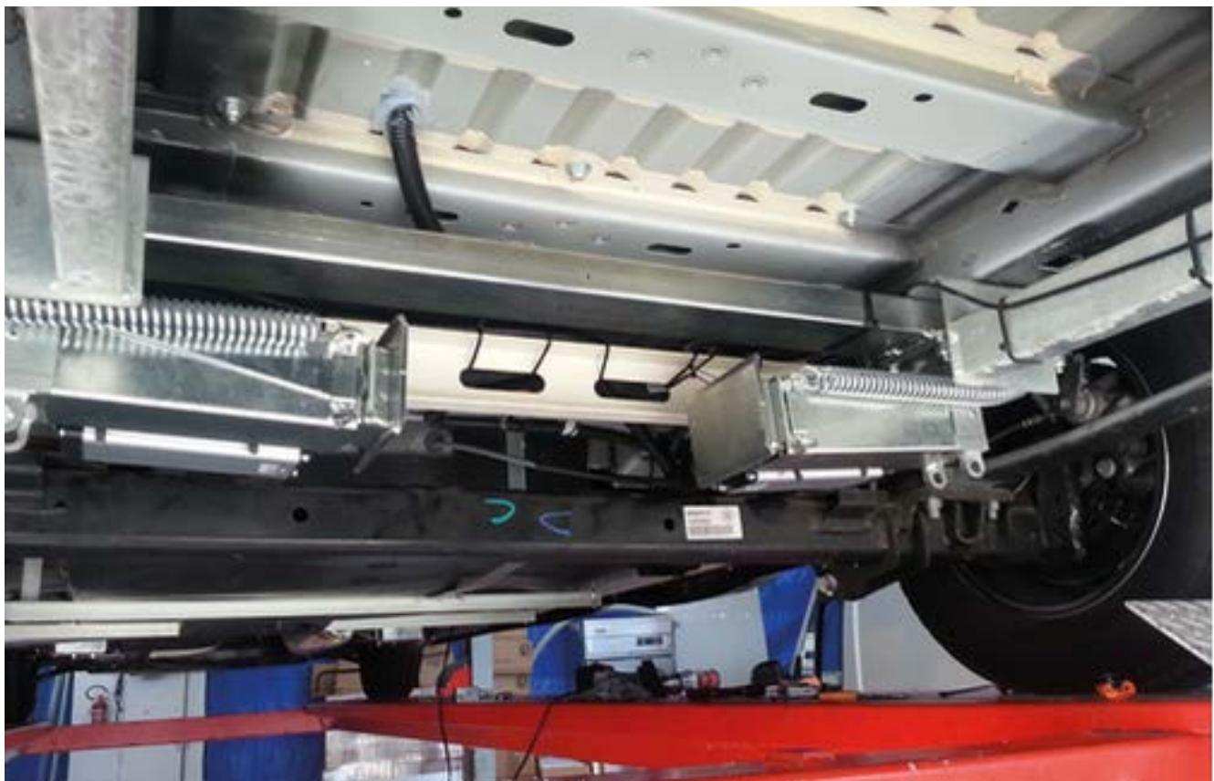
The motor jacks should be installed facing the front of the vehicle, but they have to fold towards the center.
