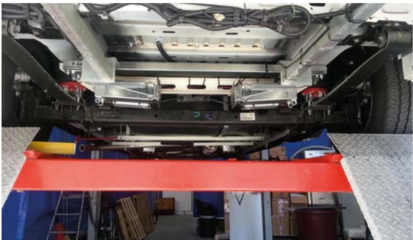
The motor jacks should be installed facing the front of the vehicle, but they have to fold towards the center.
