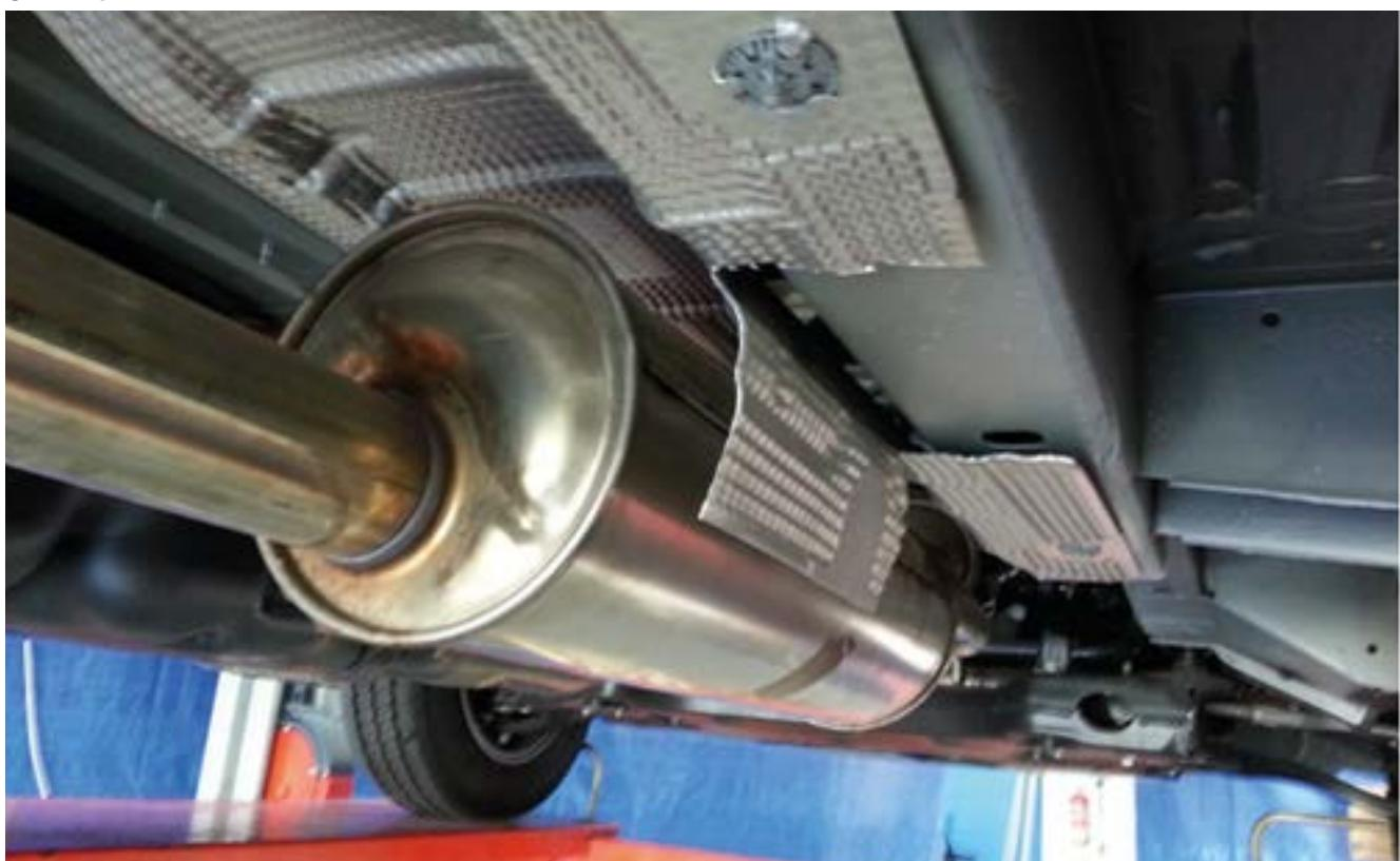
Modify the protection plate in order to create space to fix the adapter parallel to the adapter on the left.
