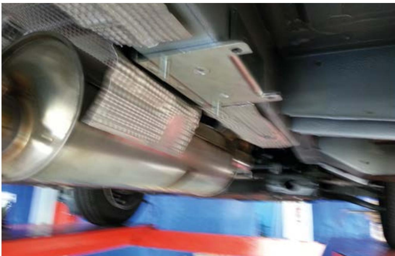
Fix the bracket to the chassis with the screws and backplate (as done on the left side).
