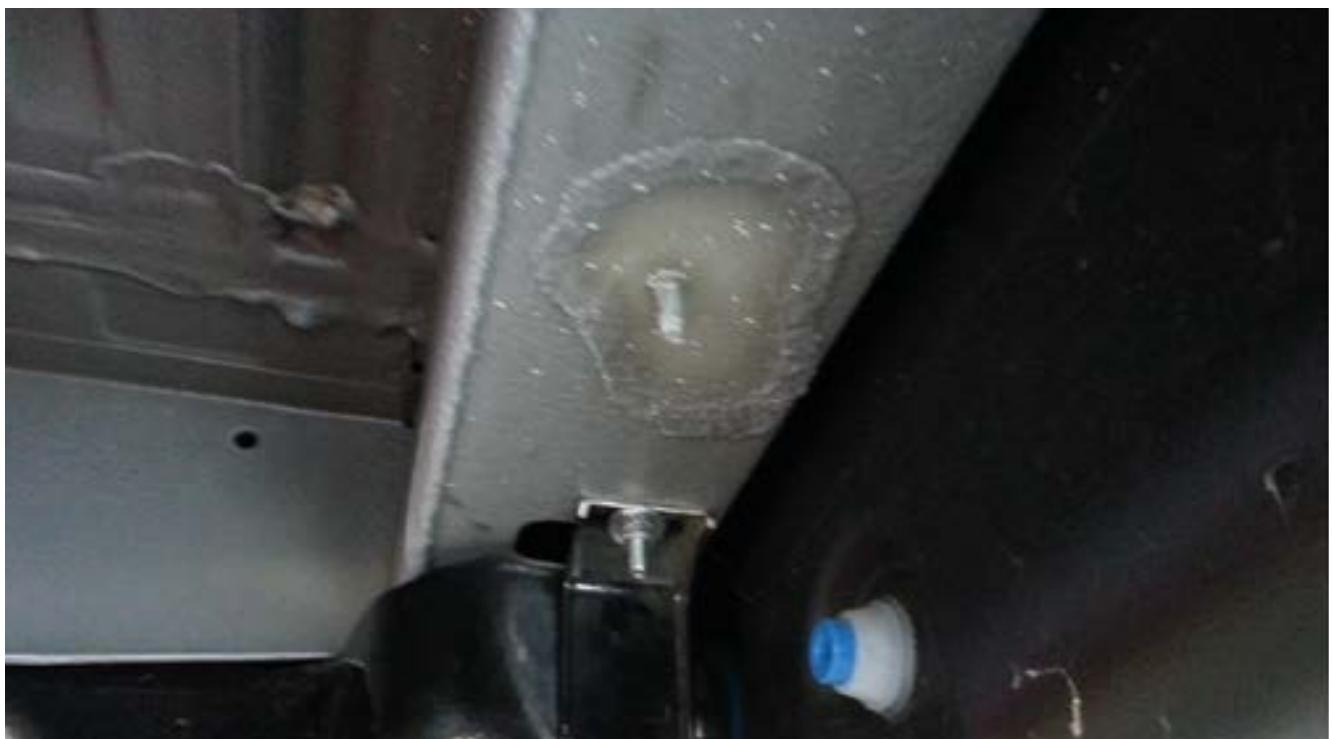
Insert the sealing plate in the hole on the frame, put the adapter and push towards the front.
