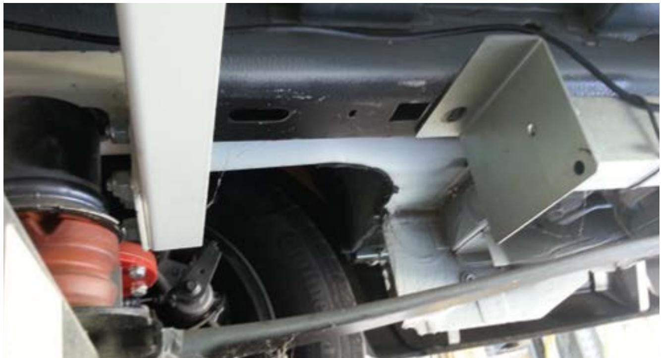
Fix the rear bracket with the square backplate: insert the backplate into the hole, then use the 12MA bolt to fix it (please see next photo).
