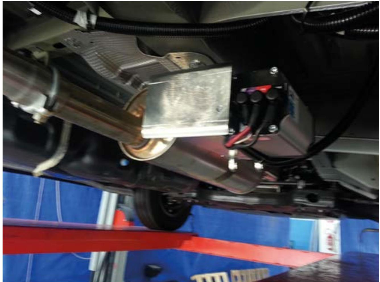
The front right jack should have the motor facing outward, while rotating towards the back.
