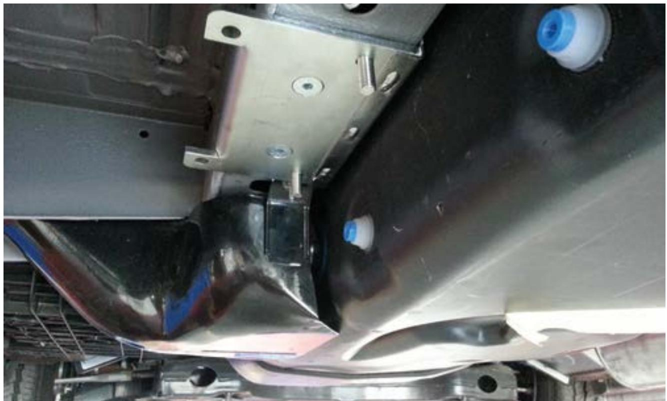
Fix the bracket to the chassis with the screws to the backplate.
