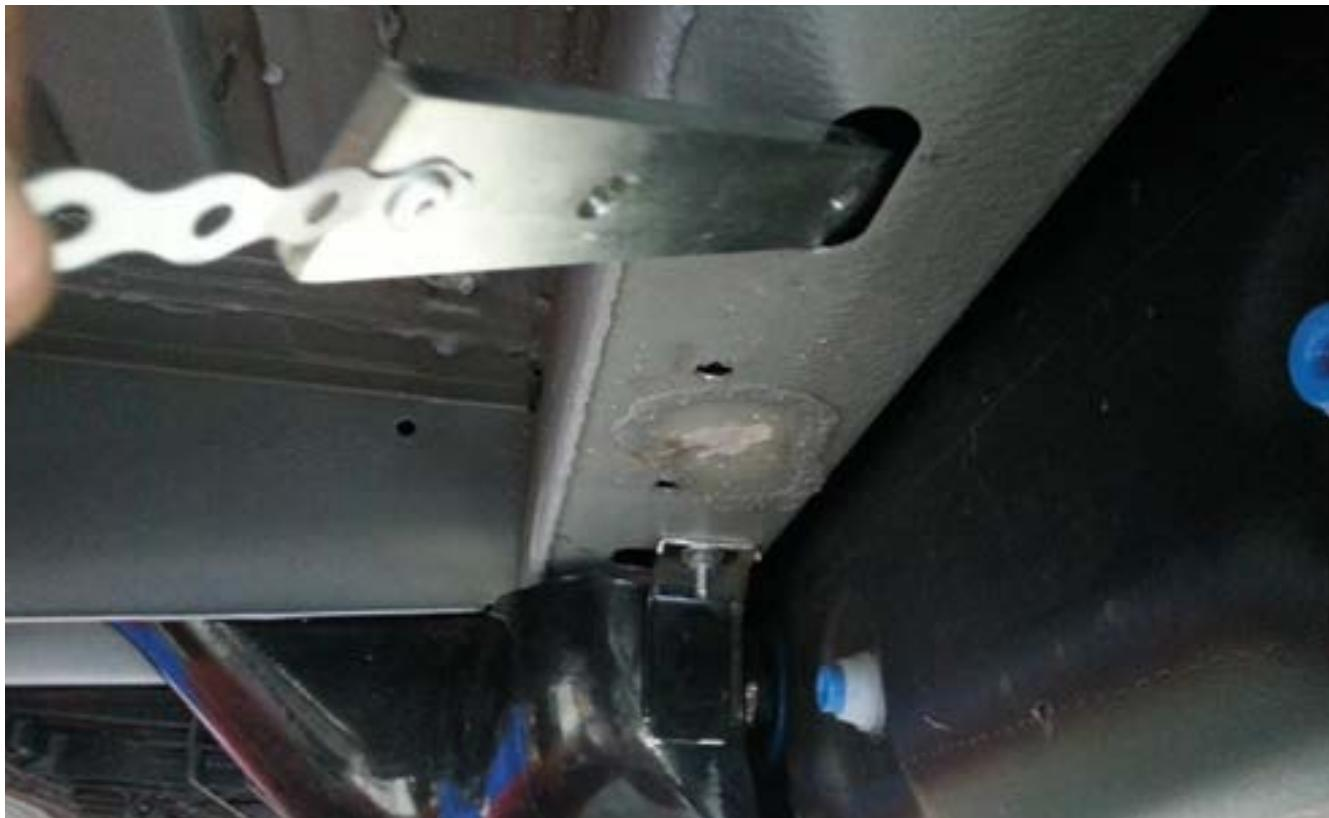
Insert the mounting backplate into the hole under the chassis.
