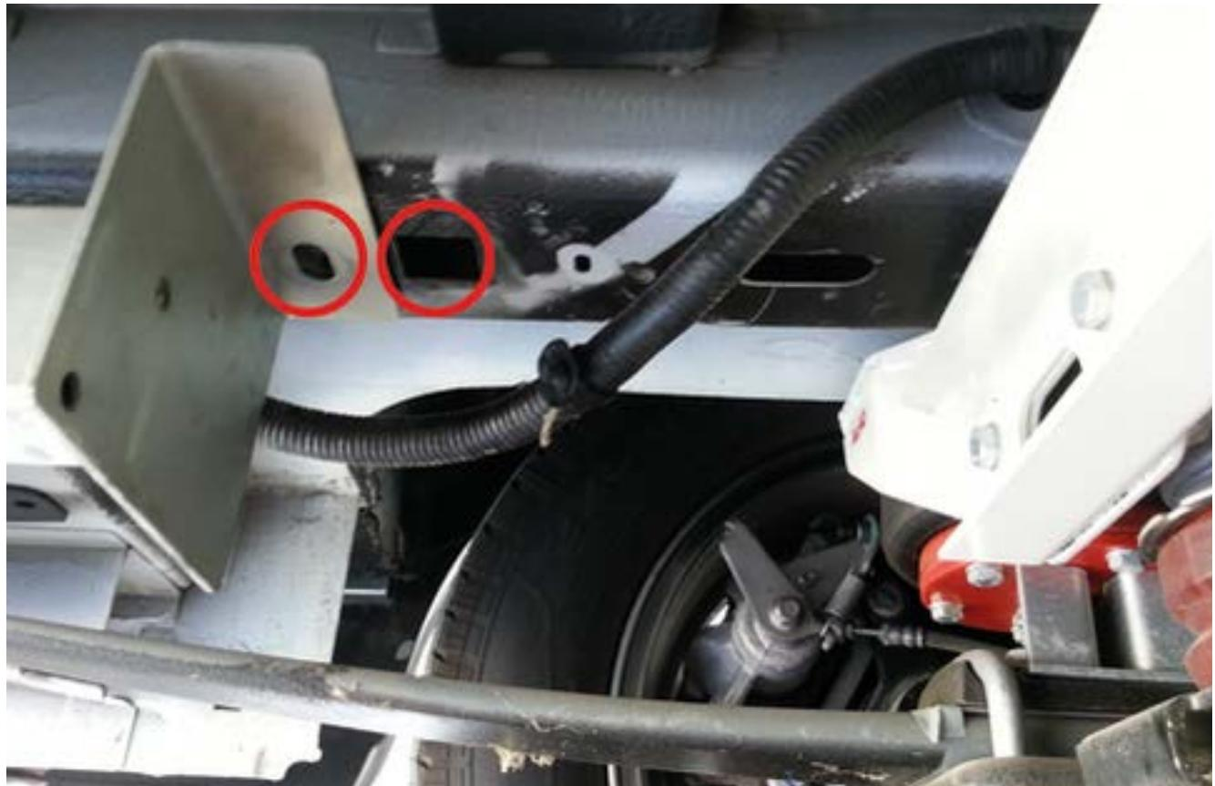
The fixing holes are pointed out in the photo.
